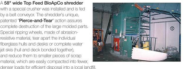
The largest hulls or decks, even when several are nested together, or complete water jet skis already filled with flotation foam, plastic ducting and metal fuel and exhaust lines, are completely destroyed in about one minute.
