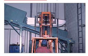
The Kawasaki Motors Manufacturing Corp. plant in Lincoln, NE, installed a giant, three-storyhigh molding press capable of exerting 3,000 tons of pressure to produce the hulls for Kawasaki water jet skis. Fiberglass sheet molding compound is molded into a top (deck) or bottom (hull) of a jet ski for three models produced at the Lincoln plant. The largest jet ski, when bonded, is about 4 feet wide, 10 feet long and 32 inches thick.
