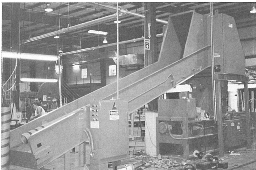
Cores being conveyed into shredder. NOTE: Shredder can be placed in-line with baler, as shown here, or 90° to baler.
